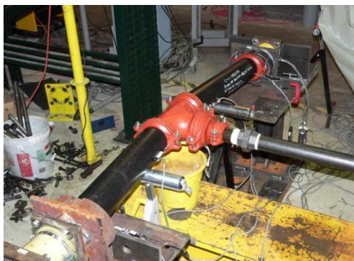
Pipe end bent due to imposed rotation
