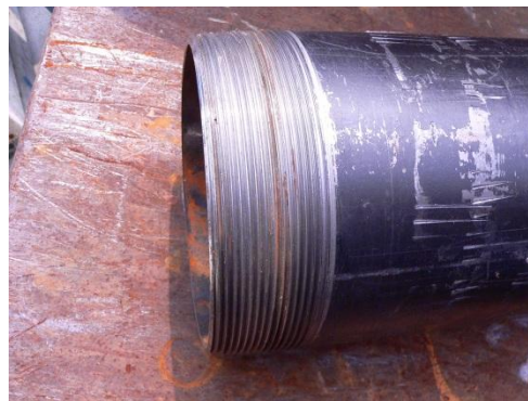
Pipe threads damage
