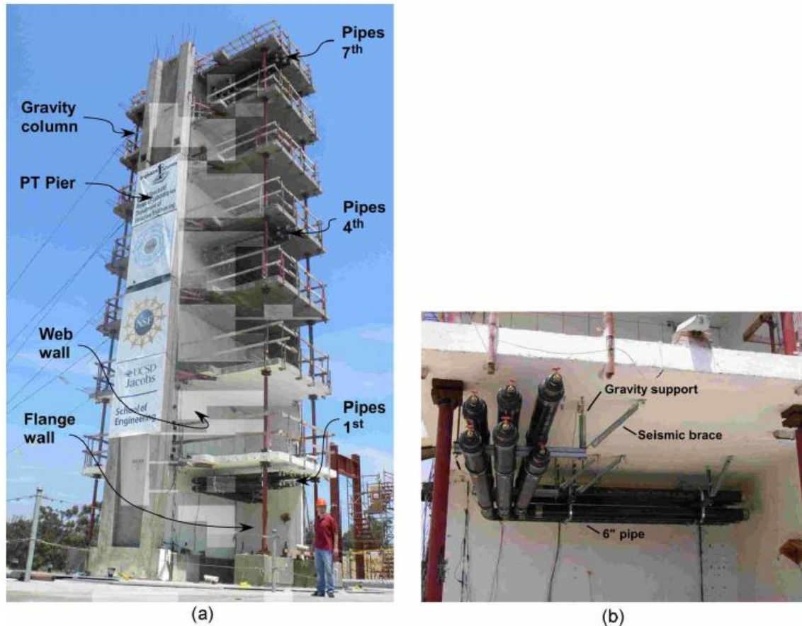
Figure 2-6 (a) Seven-story building on the shake table and (b) Nonstructural system on the first floor (from Hoehler et al. 2009)
