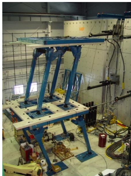
Figure 4-1 Nonstructural Component Simulator at University of Buffalo (from SEESL, 2010)
