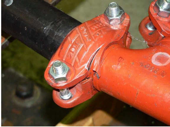
(c) Fracture of coupling flange initiated from the housing key
