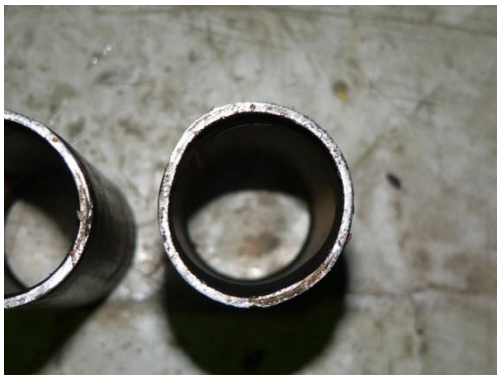
Cross section of pipe yielded and deformed
