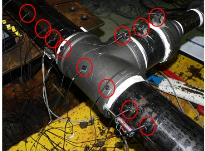
(b) LEDs attached to the piping specimen
