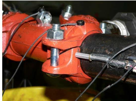
(b) Gap generated between angled pads
