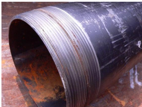
Pipe threads erode due to slippage
