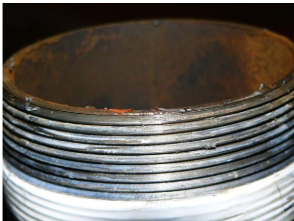
Pipe threads erode due to slippage
