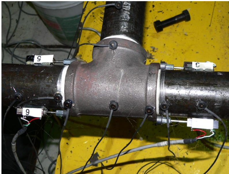
Figure 3-10 Linear potentiometers attached to a tee joint
