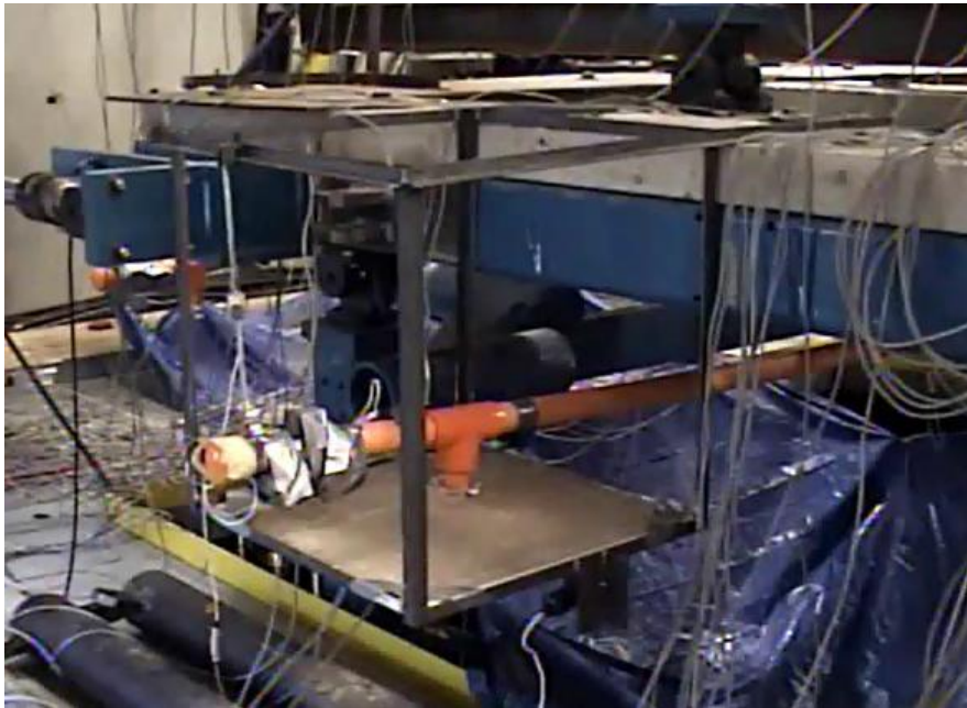
Figure 4-14 Rigid ceiling box supported by steel angles
