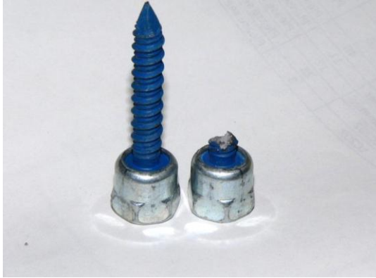
(a) SAMMY screw sheared off (Configuration 1-5, 100% MCE level)
