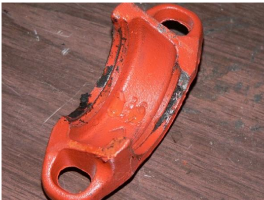
Coupling flange fractured
