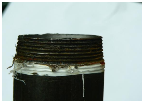
Pipe threads damage
