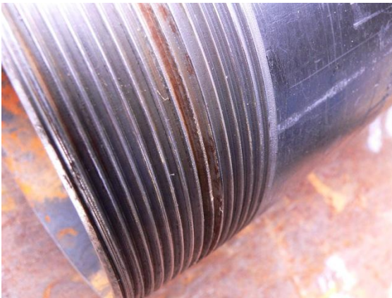
Pipe threads damage
