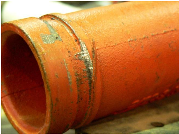
(e) Edge of groove sheared off in the tee joint
