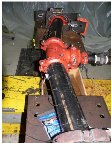
Pipe end bent due to imposed rotation
