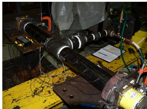
Pipe end bent due to imposed rotation
