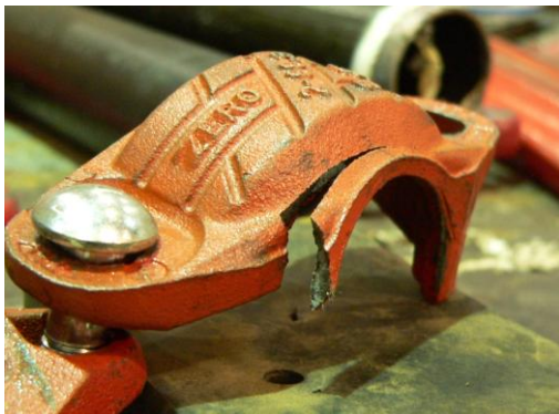
Flange coupling fractured
