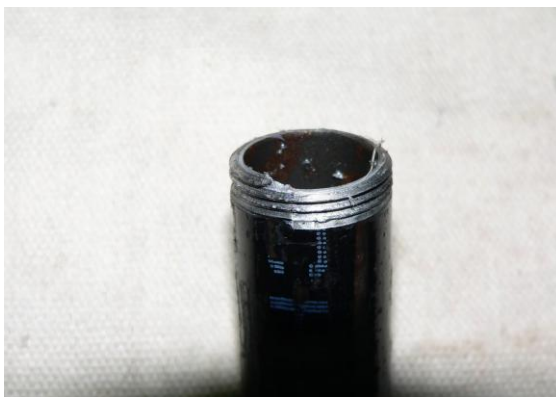
Pipe threads erode due to imposed rotation
