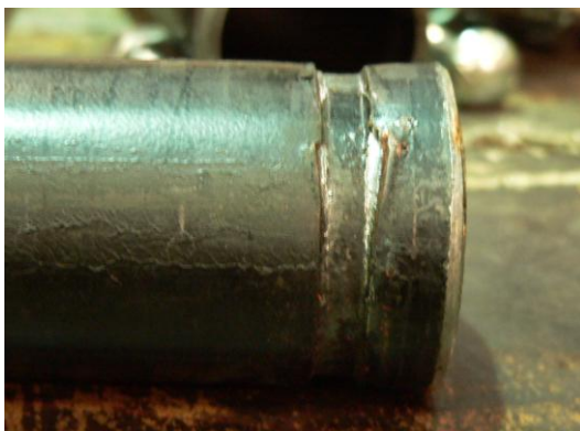
Groove of pipe wore away
