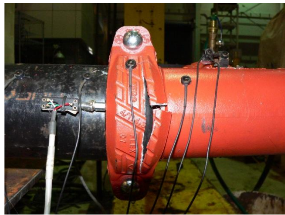
(b) Fracture of coupling flange initiated from the housing key
