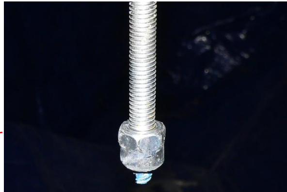
(c) Vertical hanger pulled out from concrete slab (Configuration 1-6, 100% MCE level)
