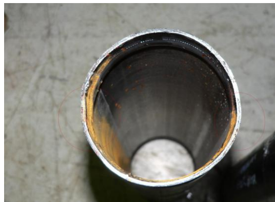
Cross section of pipe yielded and deformed
