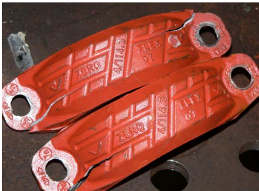
Coupling flange fractured
