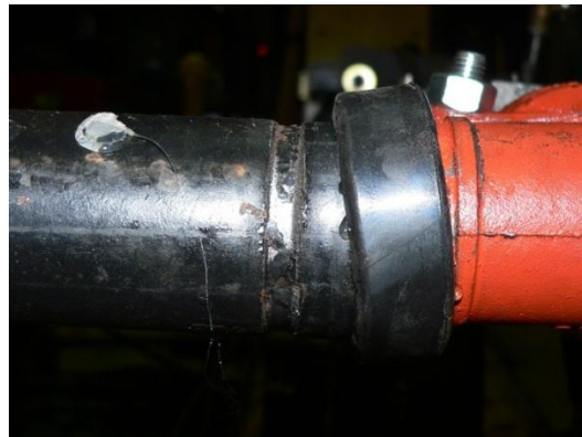
Groove of pipe wore away
