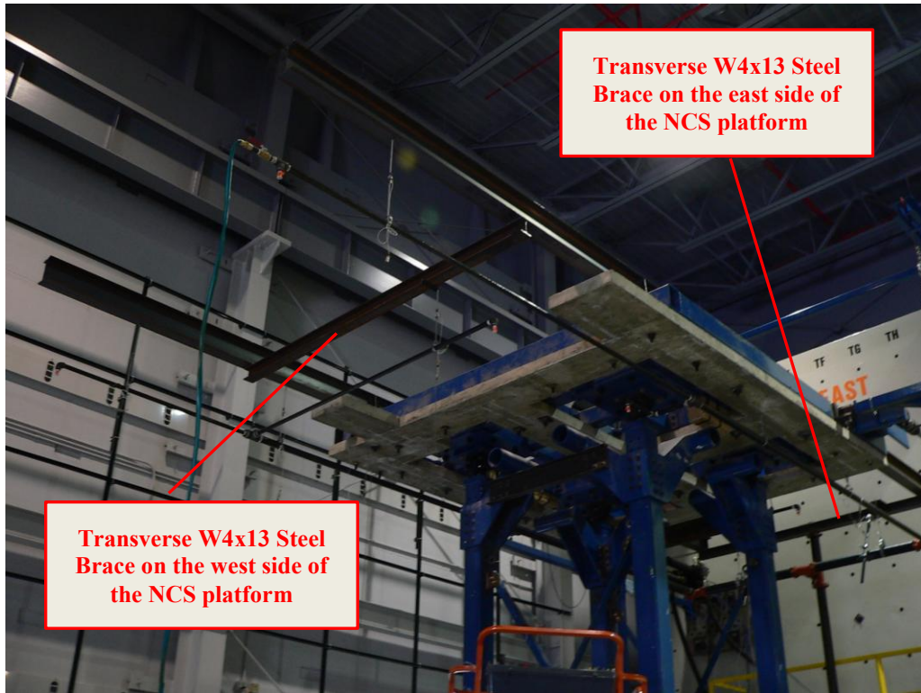
Figure 4-7 Location of steel braces for outriggers
