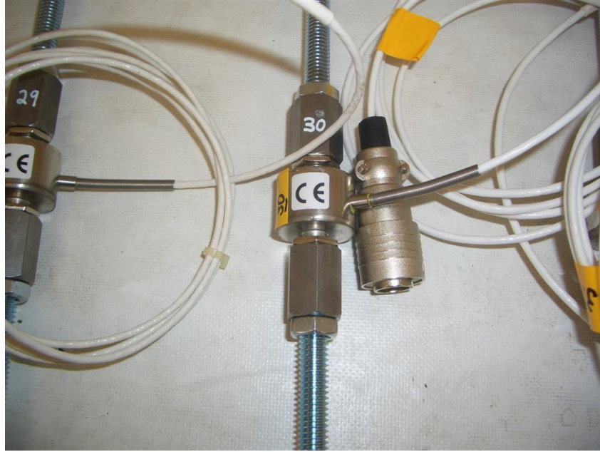
Figure 4-27 Miniature universal load cell
