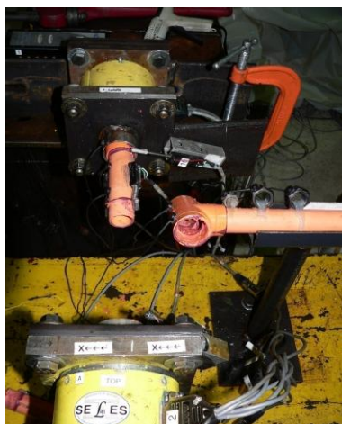
Pipe pulled out from tee joint
