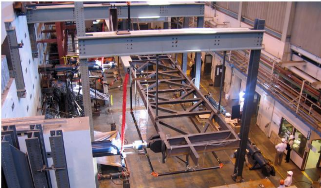
Figure 2-7 Victaulic test setup at Lehigh University's ATLSS laboratory (from Martínez, 2007)
