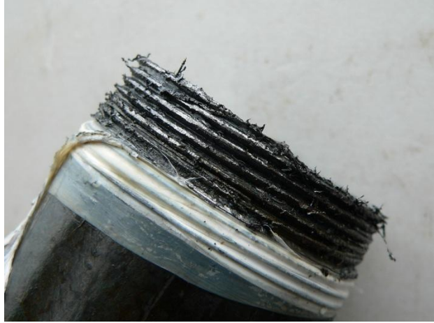
(d) Eroding of threads due to slippage
