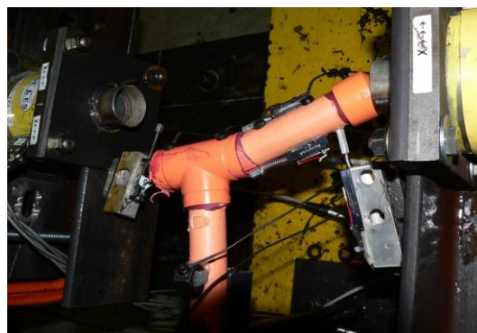
Pipe end bent due to imposed rotation
