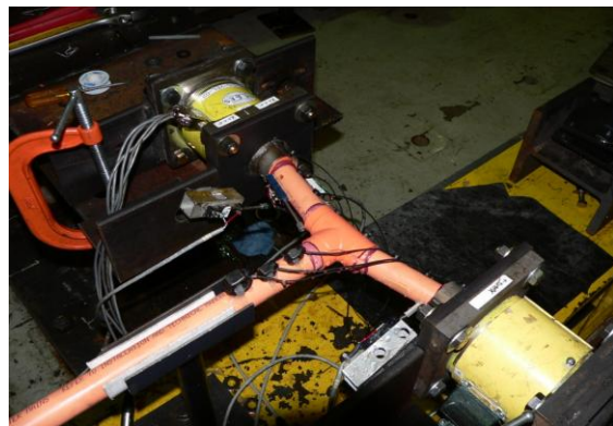
Pipe end bent due to imposed rotation
