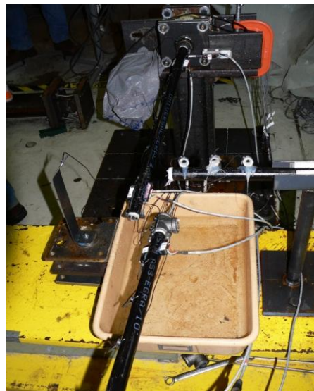
Pipe fractured at the edge of tee
