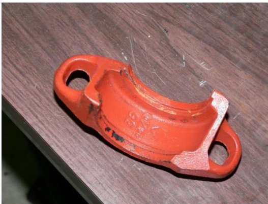
Flange coupling fractured
