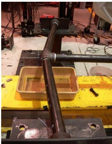
Pipe end bends due to imposed rotation
