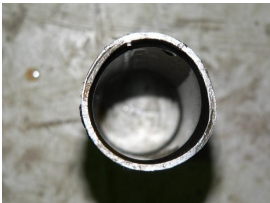
(c) Significant inelastic deformation in the pipe section
