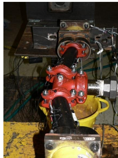
Pipe end bent due to imposed rotation
