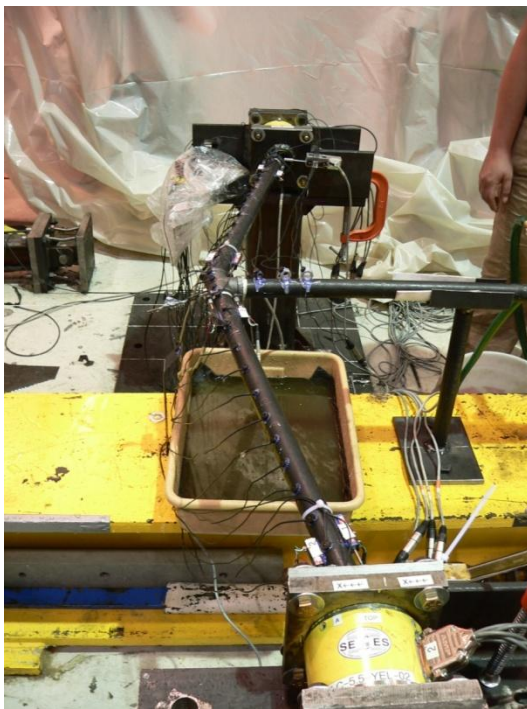
(a) Large inelastic rotation occurred at the ends of the pipes on both sides of the tee joint
