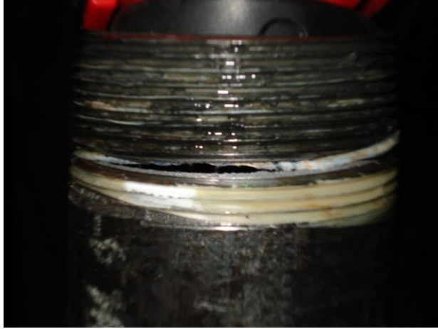
(c) Opening of threads in the pipe
